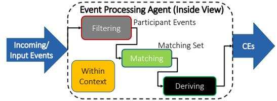
Figure 3: EPA Basic Structure.
