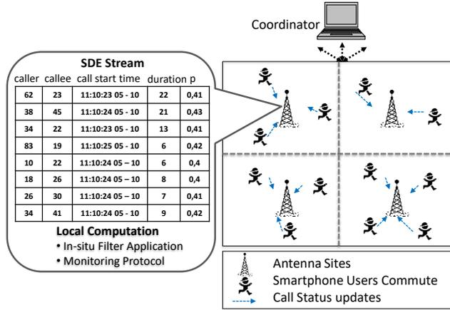
**Figure 1: An instance of site network organization into a bottom tier (telecom antennas) and a top tier (coordinator - query site). Each site applies the in-situ filter and executes the monitoring protocol proposed by our approach.**
