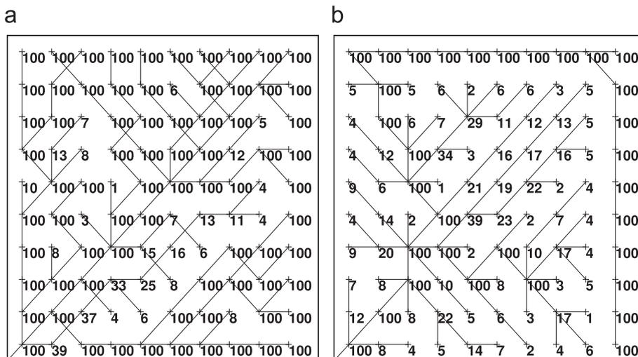
Fig. 2. (a) Collection tree for MinHops algorithm. Cost=7709 transmissions; (b) collection tree for our algorithm. Cost=3838 transmissions.
