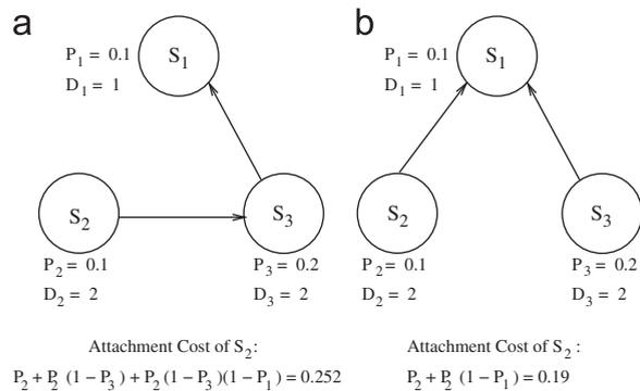
**Fig. 3.** Parent selection using the neighbor with the maximum  $P$  value leads to wrong decision in (a). In (b) the parent selection using the attachment cost leads to the best decision.
