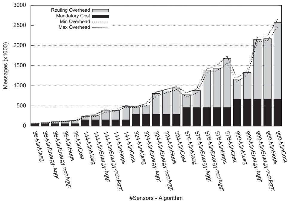
Fig. 4. Messages and average message overhead for INDEPENDENT synthetic data set. Results for `MinEnergy` presented for both aggregate `SUM` and non-aggregate query.
