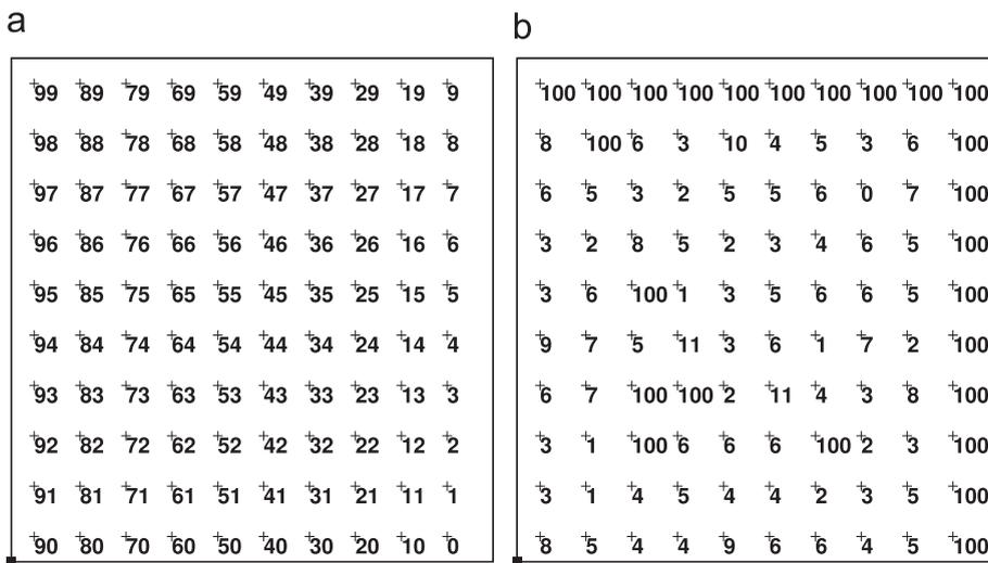
Fig. 1. (a) Identifiers of sensors in grid arrangement; (b) estimated number of participations in query result in 100 epochs.
