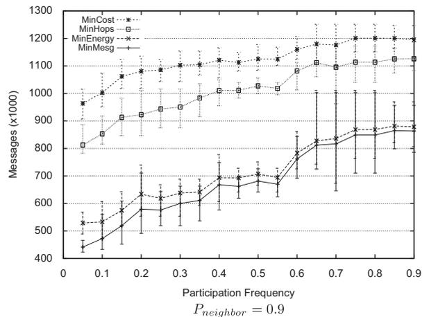
Fig. 8. Transmissions varying the epoch participation frequency, DEPENDENT setting.
