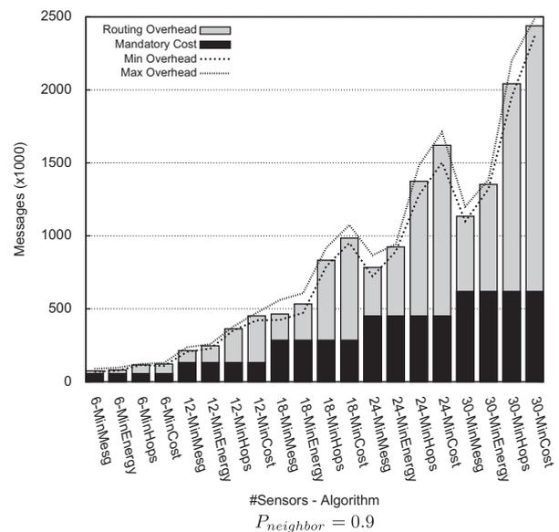
**Fig. 6.** Messages and average message overhead for SUM query in DEPENDENT synthetic data set.
