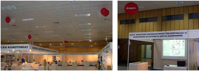
Figure 1: KSpot + 's prototype implementation deployment during the event "Researcher's Evening" at the Cyprus International Fair in 2009. (Left) Sensor nodes were placed over the pavilions using helium balloons. (Right) Sink station was connected with a laptop computer that projected the pavilions with the highest noise level.
